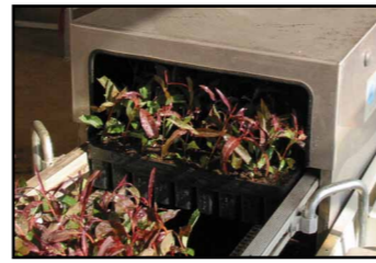
drive chain speed can be adjusted to allow for more or less water application
