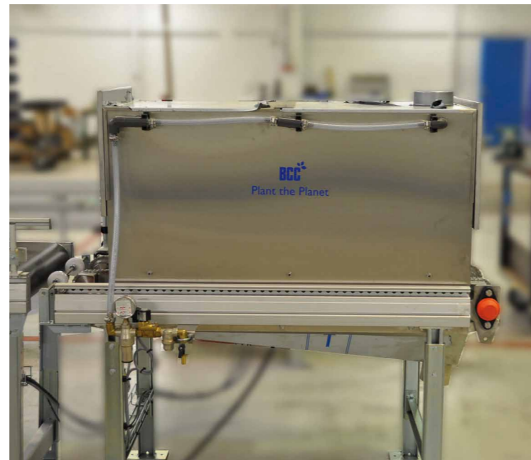
The BCC Watering Tunnel is flexible to fulfil the requirements of initial soaking, cooling through misting and application of fungicides.
