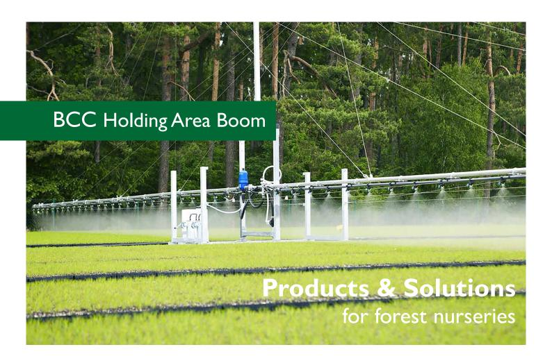
Irrigating your plants properly throughout the germination process is crucial. BCC offers customized irrigation systems for both greenhouses and holding areas. The customer can design his own irrigation system based on the needs of his specific nursery, such as dimension, irrigation features, type of nozzle, fertilizing injectors, etc
