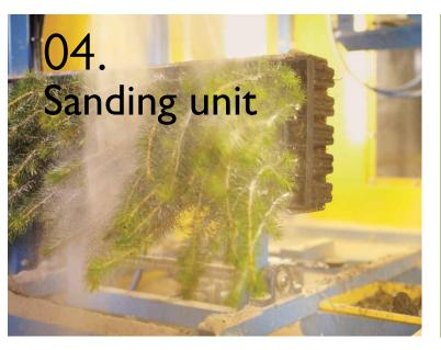
carefully fractioned, partly to counter attacks by pine weevil jaws and partly to avoid creating gaps in the protection. Surplus sand is collected in a hopper, then filtered and transported back into the system for re-use. Wet sand, needles and other particles are separated by sieving and guided to a collection vessel.
