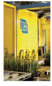
Onniflex is the new, effective and environmentally friendly coating method, protecting the forest seedling against pine weevil attacks. Conniflex as a protection method was first initiated and developed by researchers at the Swedish University of Agricultural Sciences, SLU.
